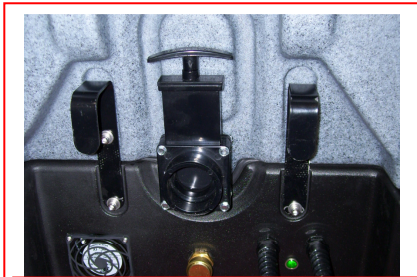
Remove four bolts holding valve assembly to flange fitting
