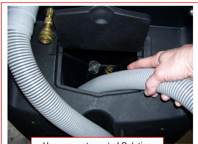
Vacuum water out of Solution Tank
