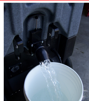
Drain water from Recovery Tank
